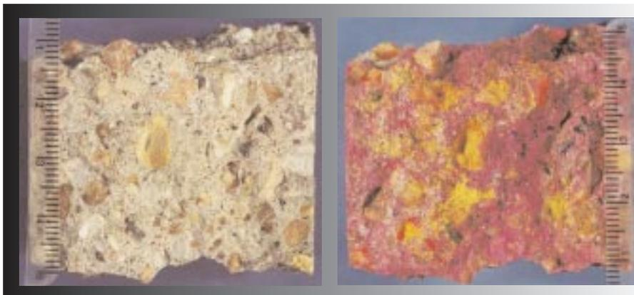
If there is no indication of ASR gel by staining and it is certain that the staining procedure was done properly, then ASR is not present in the test area. When ASR gel is indicated by a staining method, petrography and other testing must be performed.
